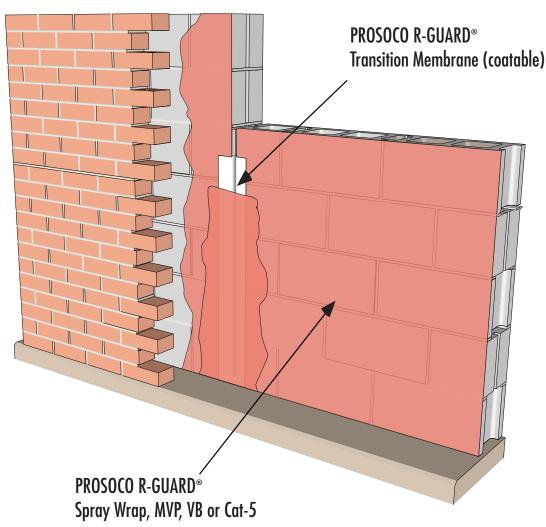
Step A. Install transition membrane Step B. Overcoat transition membrane with Spray Wrap, MVP, VB or Cat-5
