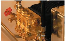
The heart of your HI FLOW 1000 Masonry Washing Machine is a heavy duty, fixed displacement pump, hand-picked to deliver 2 - 3 times as much water as conventional pressure washers. This industrial, solid shaft (24mm), 3-plunger pump is made for heavy use and lengthy service life.
